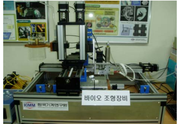
Fig. 1 RP system for 3D Scaffold
