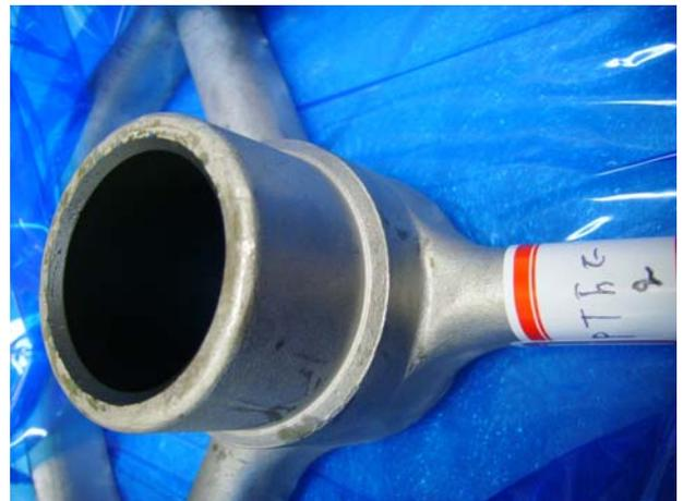
Fig. 10 Sample of teflon coated guide
