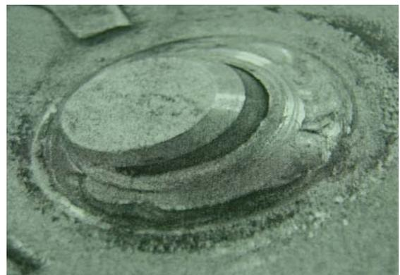
Fig. 3 Fracture of disc connection
