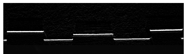
Fig. 6 Project laser stripe on calibration jigs and captured image result
