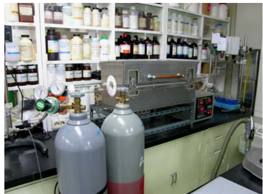
Fig. 1. Heat treatment apparatus for annealing & quenching
