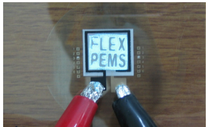
Fig. 5 EL display lamp pad-printed on a PEN film.
