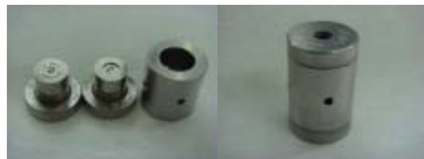
Figure 1. Photos of the mold components: upper lens core, lower lens core and bush (from left to right) and assembled mold
