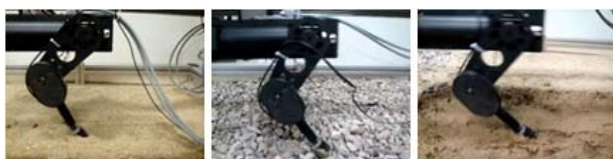
Fig.6 1-leg walking experiment on rough terrain using test bed
