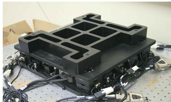
Fig. 1 4-axis nano imprinting stage
