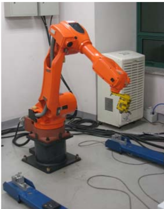
Fig. 3 HA006 and External Sensor
