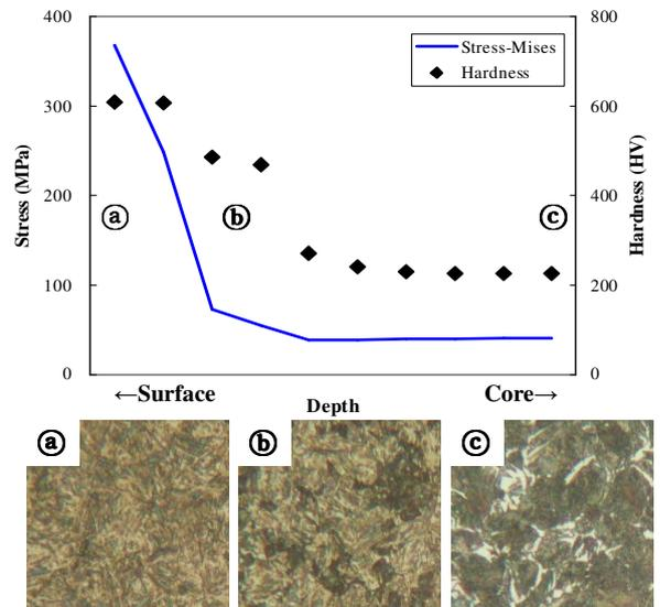
Fig. 7 Hardness(HV) and microstructure(x500); (a) Surface, (b) Boundary of hardening zone, (c) Core
