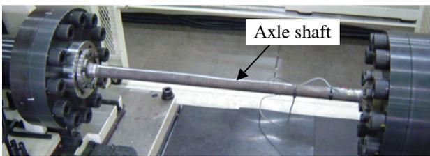
Fig. 8 Installation of Axle shaft torsion test
