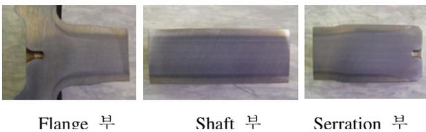
Fig. 4 Sections of induction hardened axle shaft
