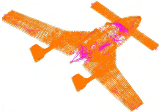
Fig. 3 Mass Modeling Results for Small Aircraft
