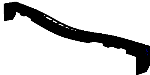
Fig. 4 Deformation of the under frame after loading
