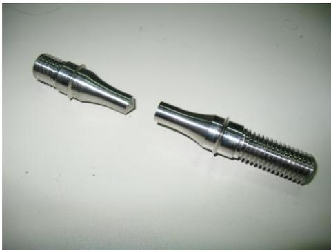
Fig. 4 Specimen for calibration
