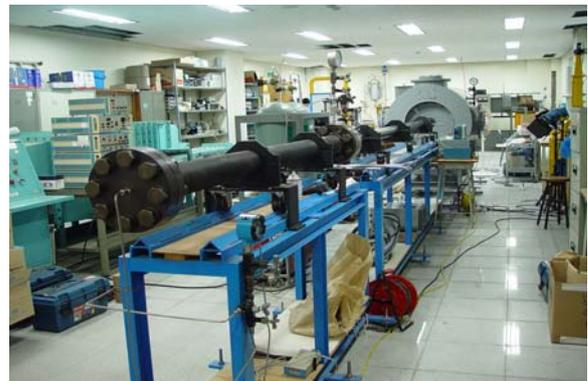
**Fig. 3** Experimental apparatus of shock tunnel
