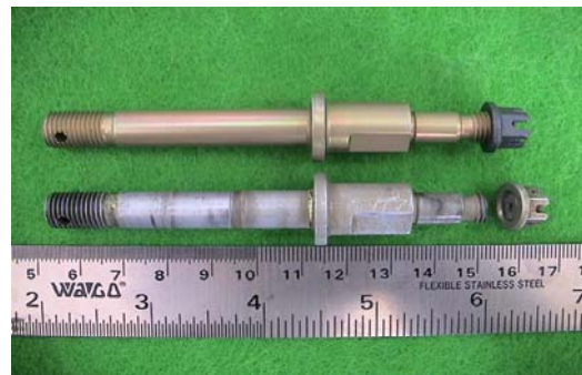
Fig. 2 Bolt failure comparison
