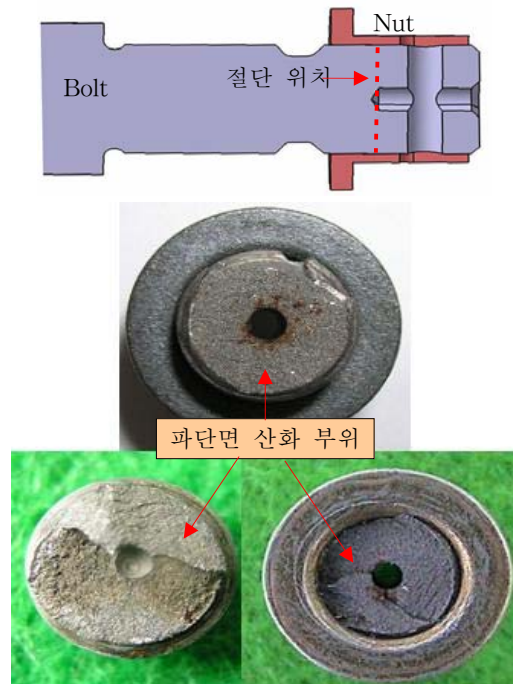
Fig. 4 Shape of rupture surface(16x, Optical microscope)
