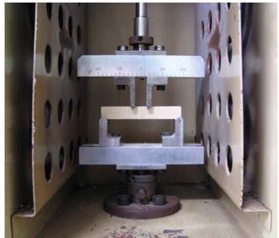
Fig. 1 Close-up view of four-point bend fixture inside the electric furnace
