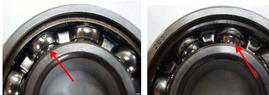
Fig. 3 Bearing cage wear in case of oil(left) and fuel(right) lubrication.
