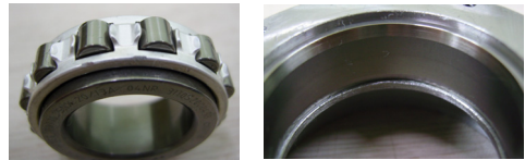
Fig. 5 Roller bearing after rig test
