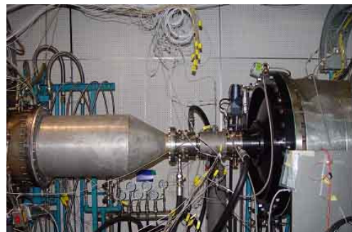
Fig. 1 Test rig for UAV engine combustor
