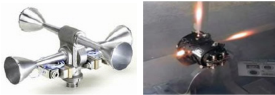
Fig. 1 Hot gas valve and thruster in DACS
