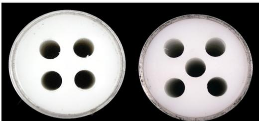
Fig. 1 Multi-port Solid Fuel Configuration
