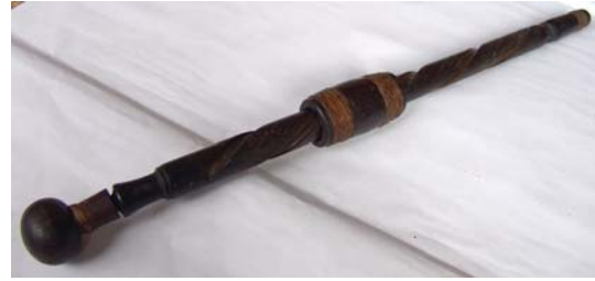
Figure 6: Primitive manual drill made from hard wood
