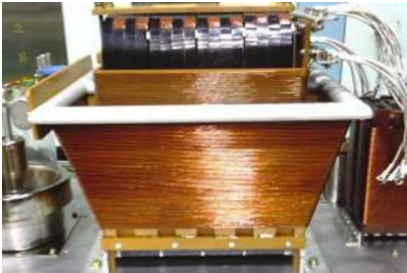
<Fig. 5> Photograph of 1:13 pulse transformer
