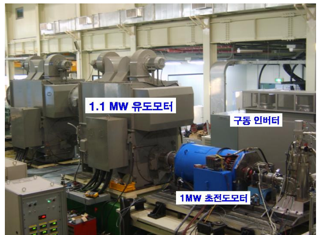
<Fig. 1> Appearance of 1 MW class HTS motor and load test facility
