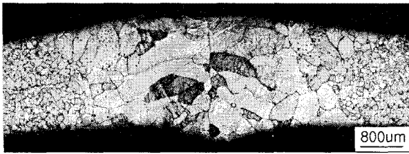
Fig.2 Macrostructure of the GTA welded STS409L-2 pipe (Grain size : 530µm)
