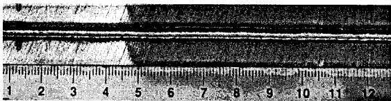
Fig. 6 Welding waveform and bead with mechanical control at 2.5m/min.(221A, 17.5V)
