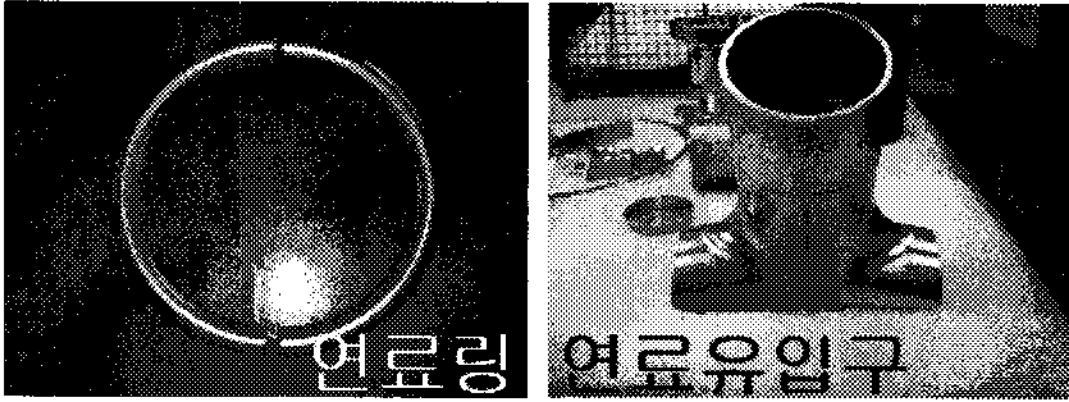
Fig. 10 Photographs of Fuel Inlet Part
