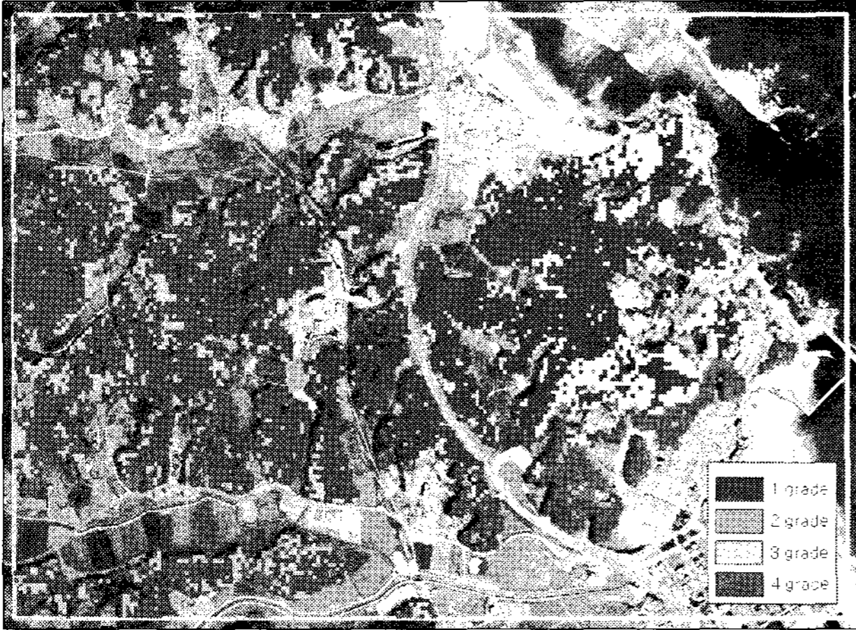
Figure 6. Grading of damaged area by forest fire
