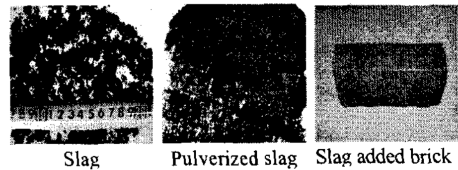
Fig. 3 Shapes of slag, pulverized slag and slag added brick
