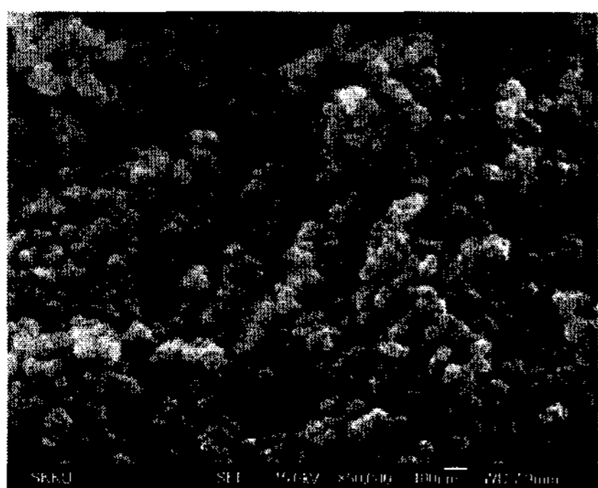
Fig. 7 FE-SEM image of used Carbon black (X 50,000)
