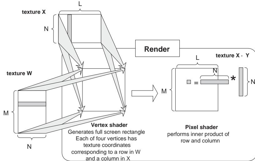
Fig. 1. Overview of matrix multiplication using GPU.
