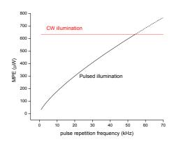
synchronized with the integration time of the high-speed line scan camera. According to the ANSI standard for safe use of lasers, the maximum permissible exposure expressed as the average power of a pulse train increases with the pulse repetition rateup to a frequency of 55 kHz, where the limit to continuous wave exposure is reached. [5]
