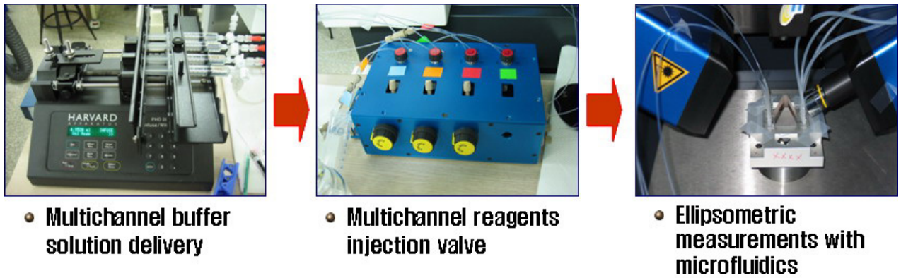
Figure : Total internal reflection ellipsometry system, (a)multi-channel buffer solution delivery system, (b)multi-channel reagents injection valves, and (c)single wavelength imaging ellipsometer
