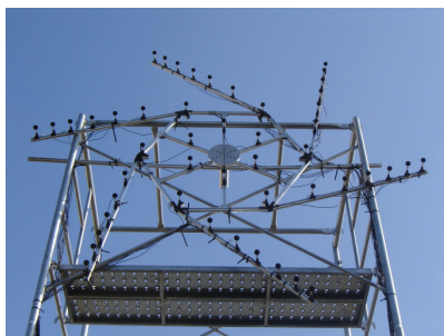
Fig. 1 Microphone array system with 48 sensors
