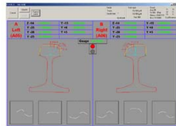
Fig.4 Example of rail profile graph compared with reference profile
