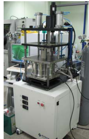
(b) Manufactured Hot Embossing System
