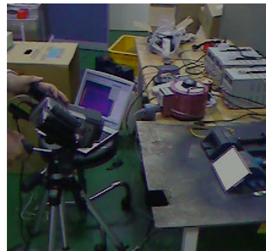
Fig.1 LCD BLU Thermal Characteristic Testing System
