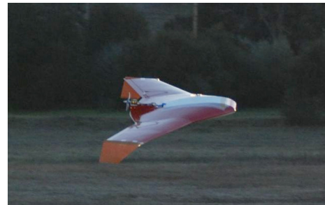
Fig. 6 Blended Wing Body-type UAV Test bed
