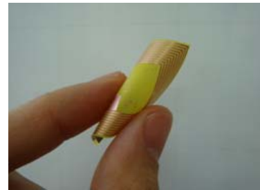
Fig.2 Optical image of fabricated air core inductor
