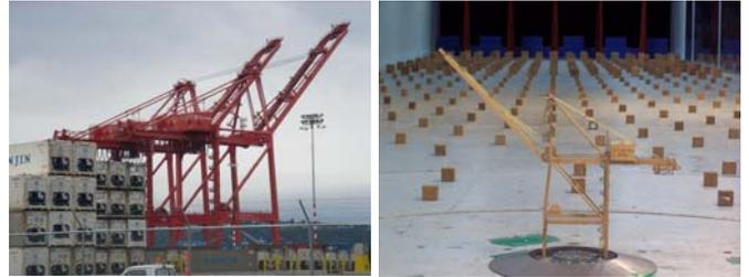
(a) Container Crane (b) Model of Container Crane
