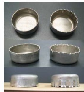
Fig. 6 Multi-stage drawing(left) vs. single stage drawing(right)
