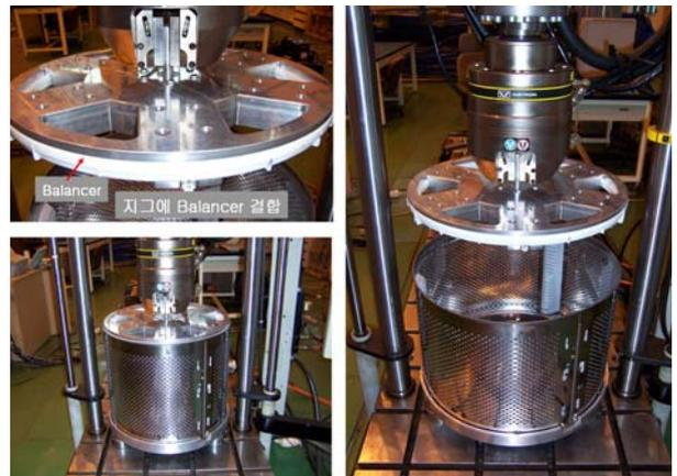
Fig. 1 Balancer and Drum connection to zig
