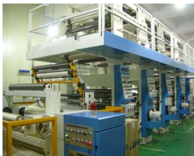
Fig. 1 Roll to roll gravure printing system
