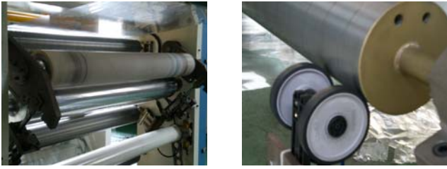
Fig. 3 Driven and idle roller in converting machine
