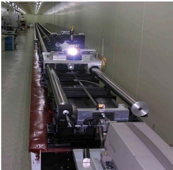
Fig. 1 Overview of the 50 m tape measuring system.
