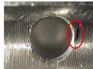
fig. 7 remaining of burr after deburring(∅2, 2000rpm, 100mm/min, 0.2MPa)
