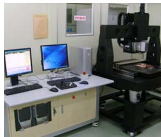
Fig.2 Photograph of 3-D measuring instrument
