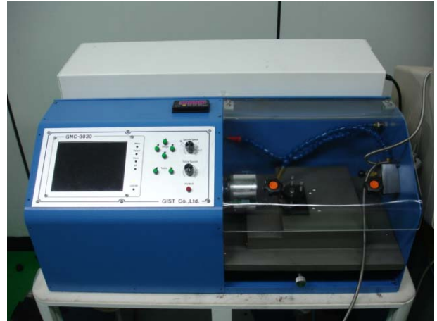
Fig. 8 The developed precision machine for fabricating micro device
