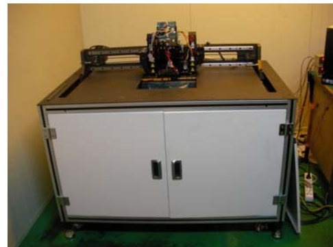
Fig. 7 8 heads 3D printing system
