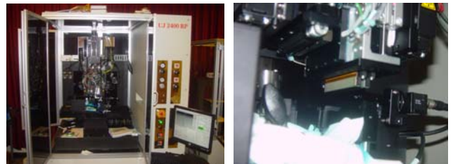
Fig. 3 2head SFF system using UV curing method
