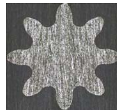
Fig. 6 Extruded gear shape
