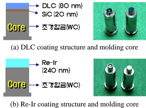
Fig. 1 Coating film structure and coated core for molding
