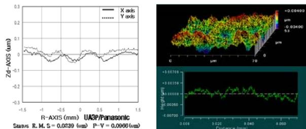
Fig. 4 Measurement of Re-Ir coating core(plane surface)
