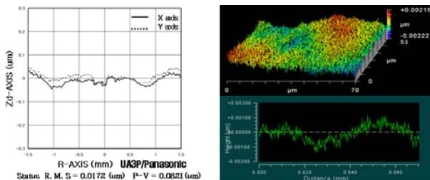
Fig. 3 Measurement of DLC coating core(plane surface)
