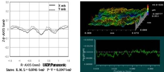
(b) Measurement of bare core for Re-Ir coating(plane surface)
