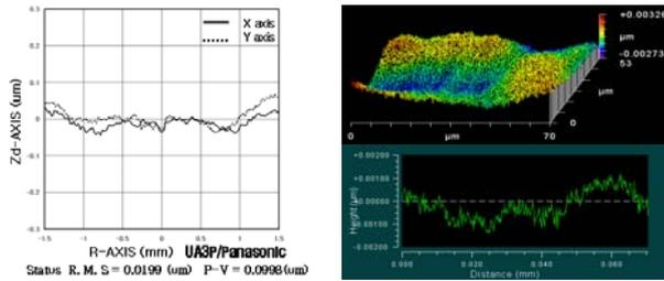
(a) Measurement of bare core for DLC coating(plane surface)
